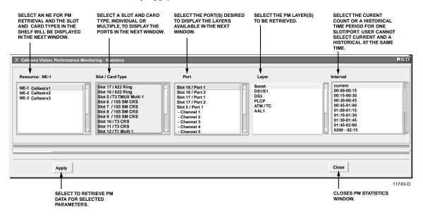
Figure 006-2. Cellworx Vision Performance Monitoring - Selection Window
